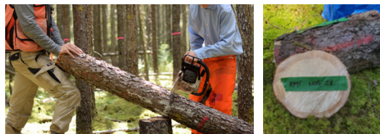
Image 2. Method 2: cutting a tree disc by felling a tree with a chainsaw. Photo by S. Dumont (2024),
