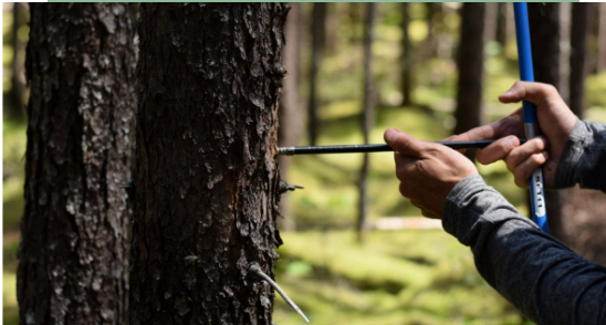
Image 1. Method 1: taking a tree core from a black spruce tree using an increment borer. Photo by S. Dumont (2024)
